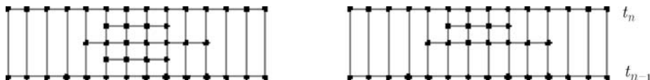
Figure 3.2: Example of a time slab created by the original strategy I (left) and the modified strategy II (right).
